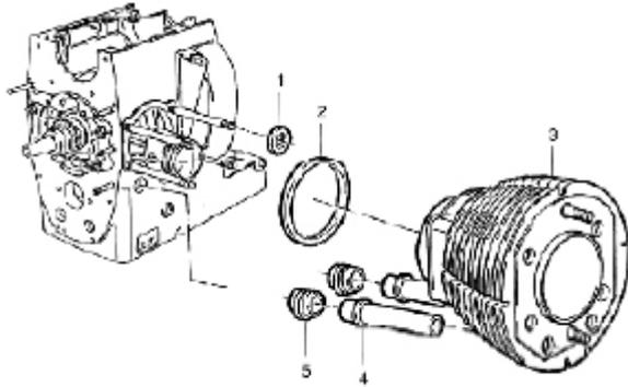
Push the pushrod rubber seals (nr. 5) on the pushrod protection tubes. Make sure the marking on the rubber is pointing outwards perpendicular to ground. Set the large O-ring (nr. 2) in to the groove on the cylinder foot.
