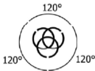
Turn the piston rings so that the opening on the second ring shows up and the other two are each shifted 120 degrees. See photo left. Press the rings together using ring compressor and insert the pistons in the cylinder up to the piston pin.
