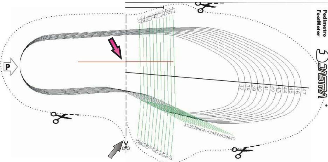
Apply together the two parts of the paper dye precisely along the cutting lines **by the care of overpositioning the axis lines (in red)**. The footMeter 1.0 is ready.
